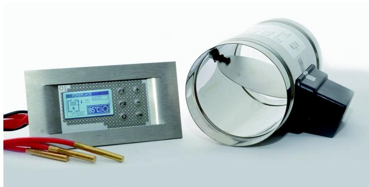
Connecting an AirSmart controller and vent is a way to avoid potential ventilation problems. A door sensor is fitted to the stove and whenever the door is opened the controller opens a sealed vent to the room to supply extra fresh air. If there is a powercut then the vent is also opened as an additional safety feature. The AirSmart controller
