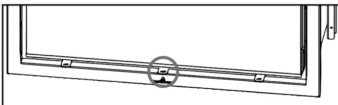
The **primary air** control lever is situated under the door in the middle. The amount of air entering the stove increases when the lever is moved in the direction of the large side of the triangular cut-out on the lever.
