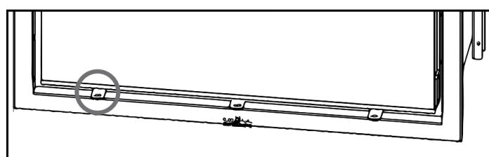
The **tertiary air** control lever is situated under the door on the left-hand side. The amount of air entering the stove increases when the lever is moved in the direction of the large side of the triangular cut-out on the lever.
