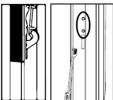
**Door closing adjustment.** On all the Octave models you can adjust the door using the bolts in the front. Tightening or loosening these bolts will ensure the correct adjustment.
