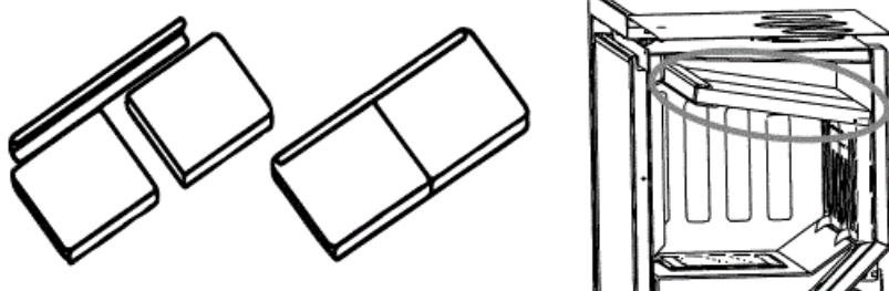
On the Octave 90i DS the baffle plate set consists of the deflector bricks and tertiary combustion tube. The RHS bricks should be positioned first, then insert the RHS end of the baffle set as far as it will go above the
