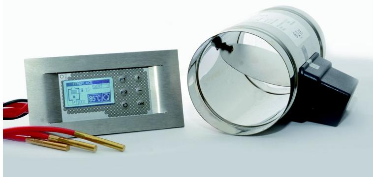
Connecting an AirSmart controller and vent is a way to avoid potential ventilation problems. A door sensor is fitted to the stove door and whenever the door is opened the controller opens a sealed vent to the room to supply extra fresh air. If there is a power cut then the vent is also opened as an additional safety feature. The AirSmart controller can be a stand-alone unit, or combined with a full automated stove
