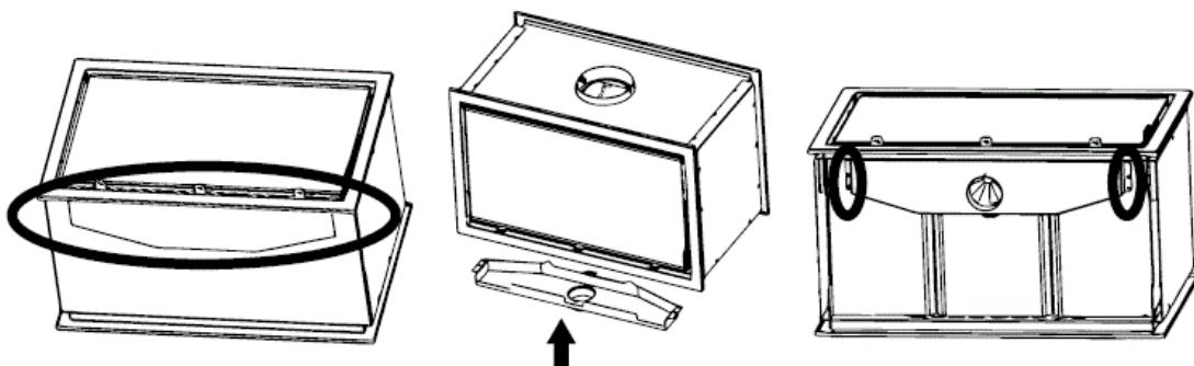
**Direct air kit for Octave 90i DS.** This optional kit enables you to bring the combustion air from the outside and will require the stove to be installed with a space underneath. This is best achieved by supporting the stove on masonry leaving space for the kit and ducting.
