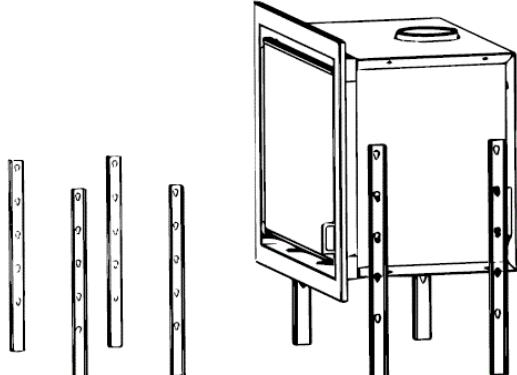
**Adjustable legs installation.** Adjustable legs are available for the Octave 70i and Octave 90i models (this option is not compatible with the Octave 90i DS) to enable the insert to be installed higher up. To fit them you must place the 4 leg holes inside the screws that you will find already screwed on both sides of the insert. You will have the choice of four different heights.
