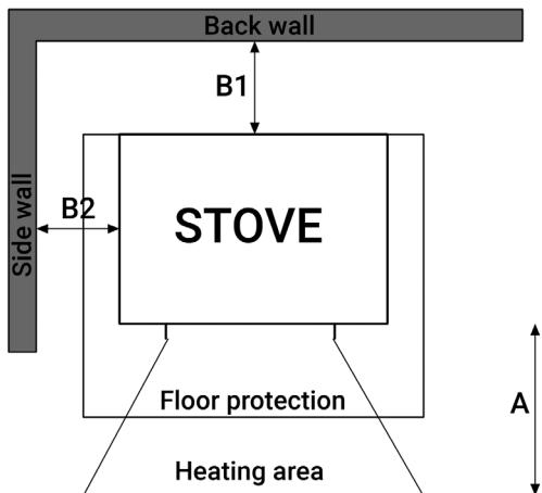
Here are the minimum distances which must be kept between the stove and combustible walls and other combustible materials.
